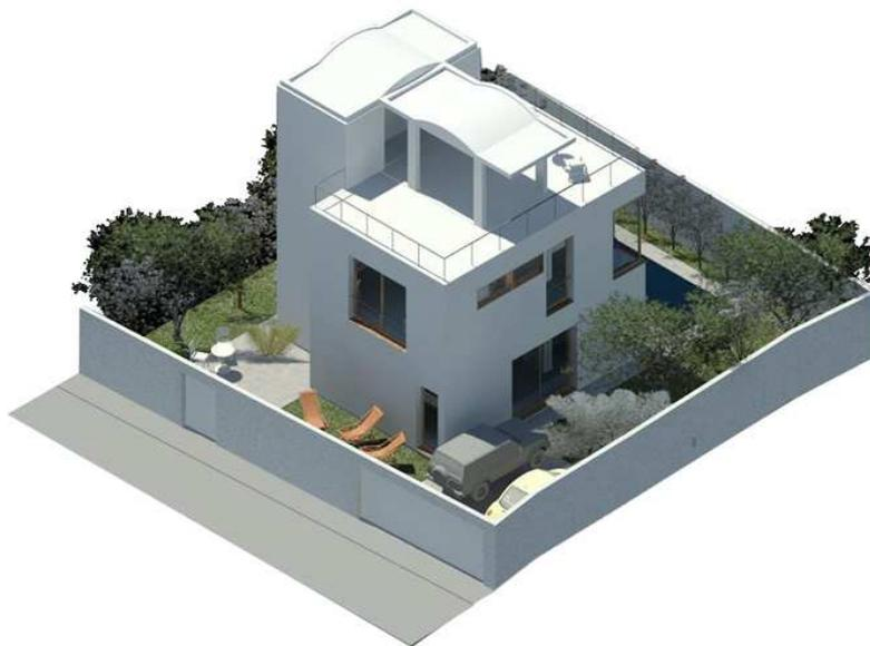
The work programme includes the manufacturing of 11 modules and a concrete platform for the terrace. The finishing process will follow according to the architectural specifications and finishing details of the client as specified in the housing project and in accordance with the Technical Code of Buildings
